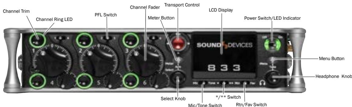
**CHANNEL TRIM** Turns the channel on/off and sets the input gain for the channel. To conserve power, turn off unused channels by rotating channel trim fully counter-clockwise.
