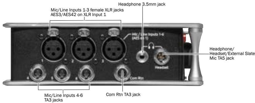
**INPUTS 1-3 FEMALE XLR JACKS** Active-balanced analog microphone or line-level inputs. Input 1 can also accept AES3 or AES42 signal. [pin-1 = ground, pin-2 = hot (+), and pin-3 = cold (-)].
