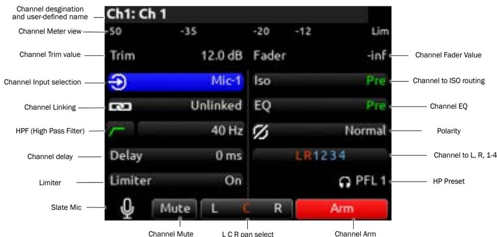
**CHANNEL DESIGNATION AND USER-DEFINED NAME** Indicates mixer channel and user-defined name. Both are overlaid onto the channel audio meter. When in a Channel Screen, hold the PFL Switch for about 0.5 s to enter the virtual keyboard and enter a user-defined name for the channel.
