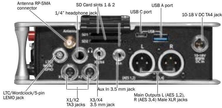
**ANTENNA RP-SMA-MALE CONNECTOR** Connects to included external antenna for Bluetooth LE.
