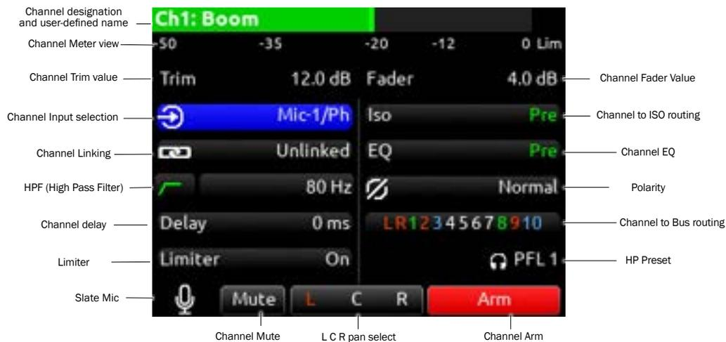
**CHANNEL DESIGNATION AND USER-DEFINED NAME** Indicates the mixer channel designation and the user-defined name. Both are overlaid onto the channel audio meter. When in a Channel Screen, hold the PFL Switch for about 0.5 s to enter the virtual keyboard and enter a user-defined name for the channel.
